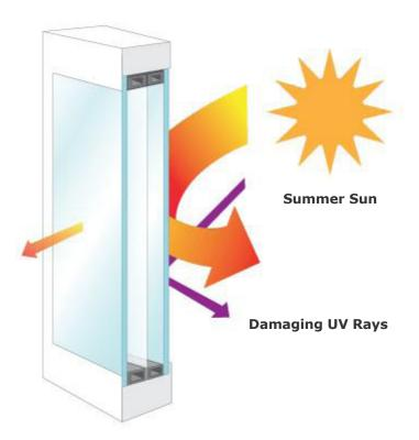
Alpen Windows low-E coatings reflect excess solar heat back outside in the summer and block harmful UV rays
