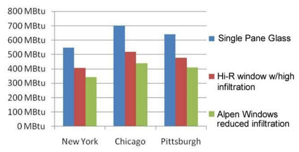
As the graph above highlights, R-value and air infiltration both contribute incremental improvements to the overall energy usage. While absolute energy consumption varies somewhat among the cities, the upgrade from single pane, low R-value, high air infiltration windows to high R-value low air infiltration windows created savings in energy consumption across the board.
