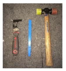
1.) Start at center of Jamb/Head/Sill. Insert 5-in-1 Painters tool between the glazing bead and the window frame. Gently lever the tool away from the frame to release the glazing bead (being careful not to damage the finish).
