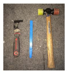
1.) Carefully wedge the Five-in-One Painters tool (with the pointed tip up & being careful not to damage the finish) between the glazing bead and frame at the top of the piece you are releasing from the window frame. The glazing bead has a lip/groove on it that is wedged into the frame and allows the glazing bead to snap into a channel on the frame when pressure is applied to it.
