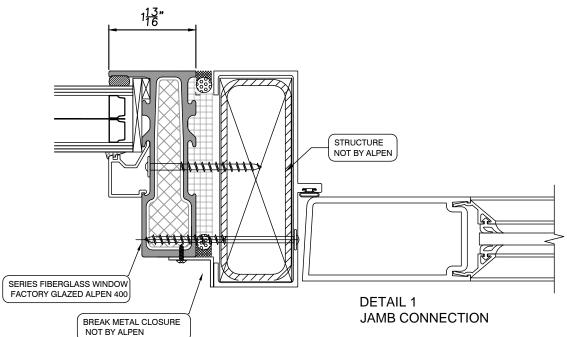
ADJUSTIBLE REDI-FLEX STEEL FRAME OR SIMILAR OVER FRAMING TO SUPPORT RIBBON WINDOW AND DOOR FRAME
